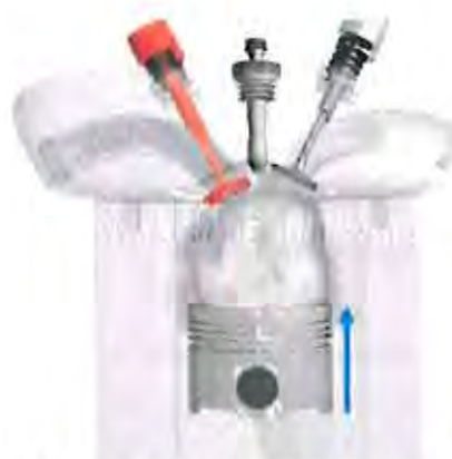
Figura 4.11. Evacuarea la motoarele Diesel (Sursa: Learn Engineering).
