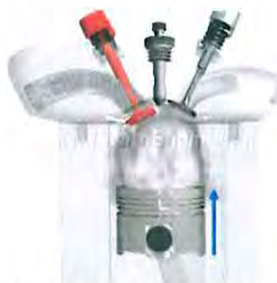
Figura 4.11. Evacuarea la motoarele Diesel (Sursa: Learn Engineering).
