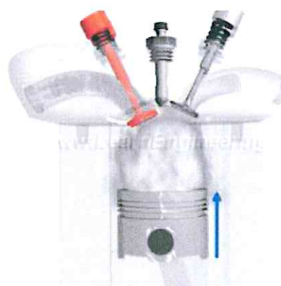
Figura 4.11. Evacuarea la motoarele Diesel (Sursa: Learn Engineering).
