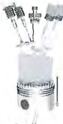
Figura 4.8. Admisia la motoarele Diesel (Sursa: Learn Engineering).
